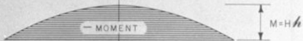
HORIZONTAL-THRUST MOMENT ( P = 0 )
