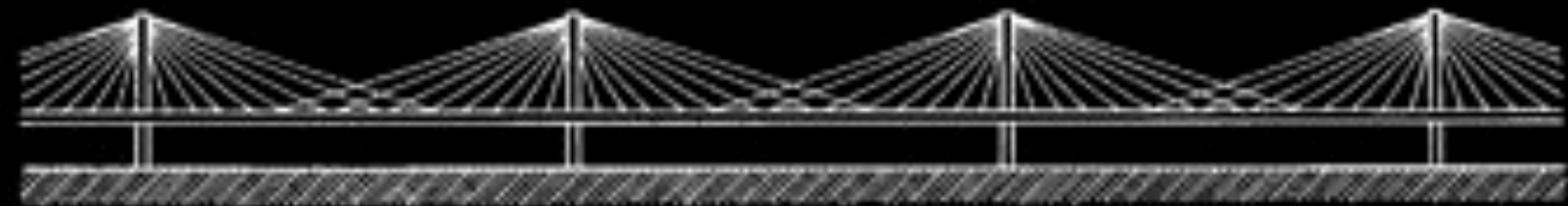
d. Cable-stays coming from both adjacent pylons to support the central part of each span.
