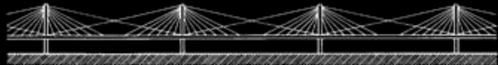
c. Long cables from a pylon head to an adjacent pylon at the deck level.
