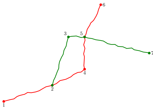
Fig. 10. Dual-line network: 2 lines (1–2–4–5–6 and 2–3–5–7), 7 edges, 7 vertices, 2 faces; \{l, m, n, r\} = \{2, 7, 7, 2\} .
